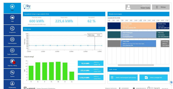
Sky Light system home page - current information on: energy consumption, saving, power consumption
