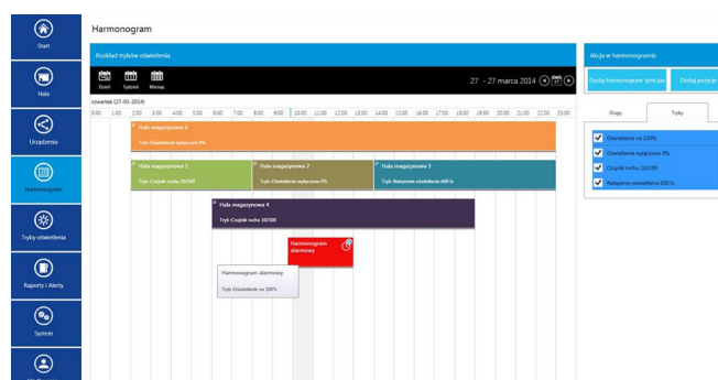
SkyLight lighting system work schedule
